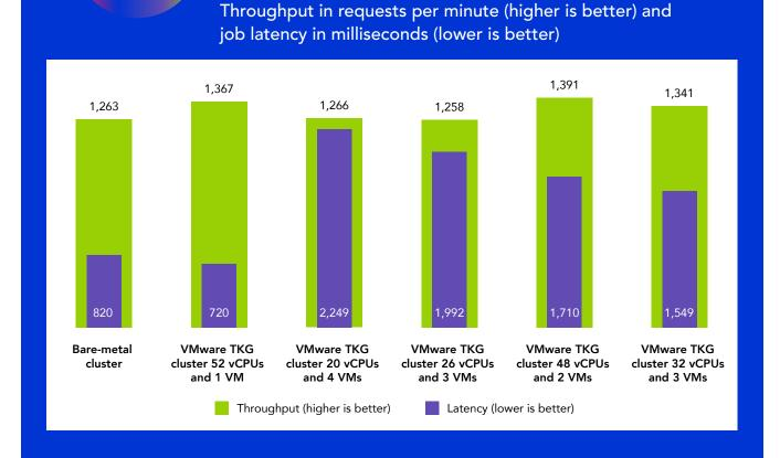
Figure 2: CloudXPRT web microservices workload results for the two clusters. Higher throughput rates and lower latencies are better. Source: Principled Technologies.
