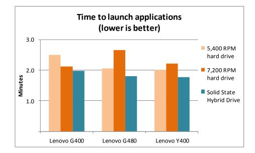
Figure 1: The laptops with the Seagate SSHDs launched applications more quickly than those with HDDs. Smaller numbers are better.
