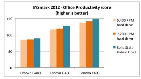
Figure 7: The SYSmark 2012 Office Productivity scores of the laptops with the Seagate SSHD were consistently higher than those of the laptops with the spindle drives.
