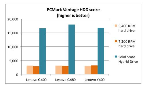
Figure 5: The PCMark Vantage HDD Scores of the laptops with the Seagate SSHD were as much as 503.3 percent higher than those of the laptops with the spindle drives.
