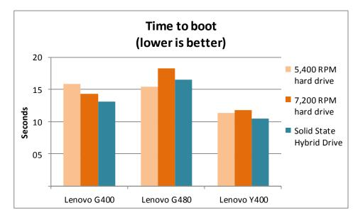
Figure 3: The laptops with the Seagate SSHDs booted more quickly than those with HDDs. Smaller numbers are better.
