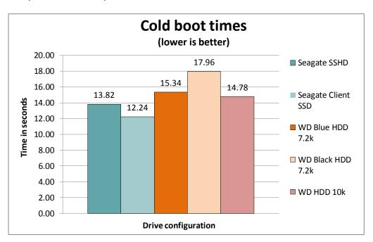
Figure 1: The desktop with the Seagate SSHD booted more quickly than with HDDs and comparably to the Seagate Client SSD configuration.
