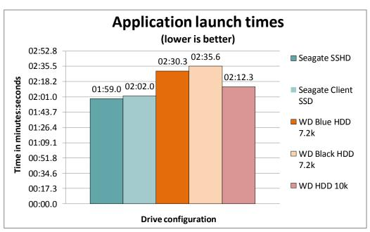
Figure 3: The desktop with the Seagate SSHD launched applications more quickly than with HDDs and the Seagate Client SSD. Smaller numbers are better.
