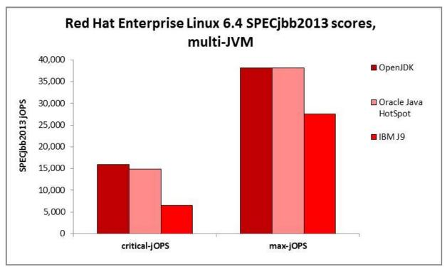
Figure 3: Multi-JVM SPECjbb2013 results comparison.
