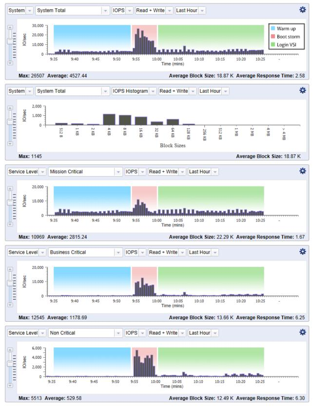
Figure 37: NexGen N5 interface showing IOPS generated during testing.
