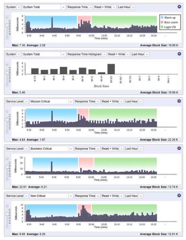
Figure 38: NexGen N5 interface showing response times during testing.
