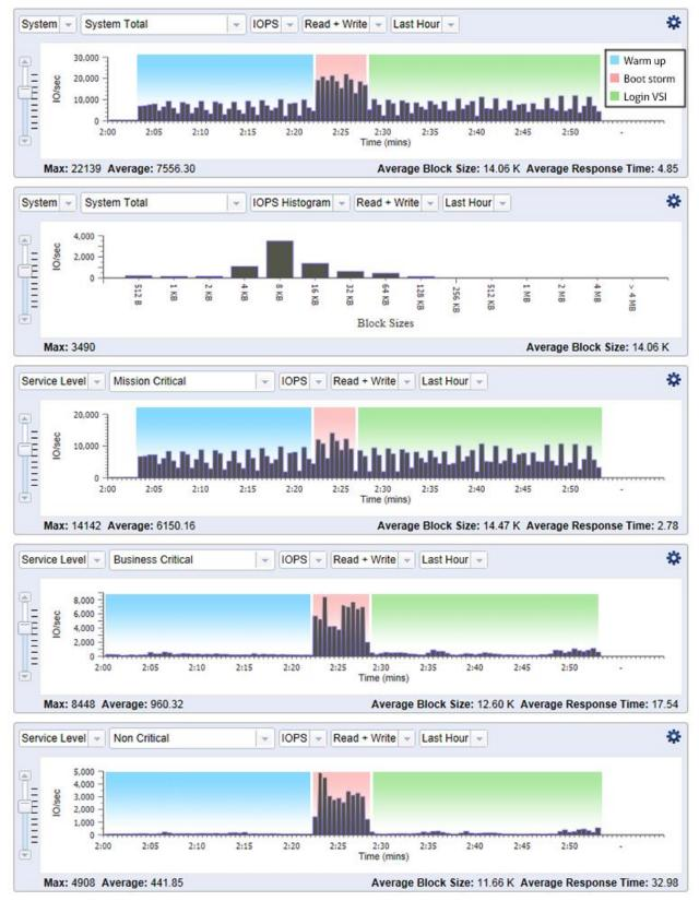
Figure 46: NexGen N5 interface showing IOPS generated during testing.
