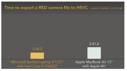
Figure 3: Time, in minutes: seconds, to export a RED camera 8K 1.5GB file to HEVC (H.265) in Adobe Premiere Pro. Lower is better. Source: Principled Technologies.
