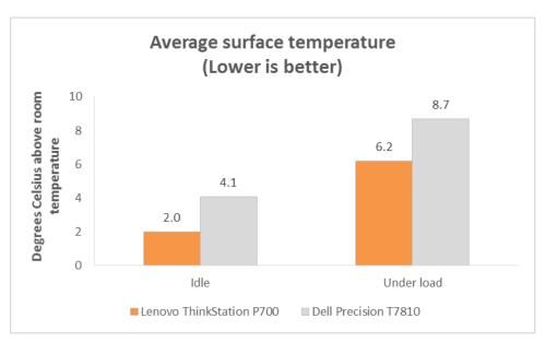
Figure 2: When idle and under load, the Lenovo ThinkStation P700 ran cooler than the Dell workstation.
