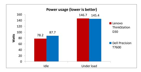
Figure 3: When idle, the Lenovo ThinkStation D30 used 10.8 percent less power than the Dell workstation.
