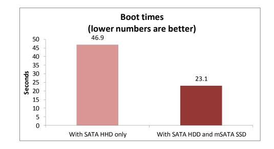
Figure 2: When we added an mSATA SSD, the Lenovo ThinkStation C30 booted 50.7 percent faster than when it used only a SATA HDD.
