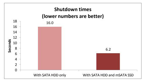
Figure 1: When we added an mSATA SSD, the Lenovo ThinkStation C30 shut down 61.5 percent faster than when it used only a SATA HDD.
