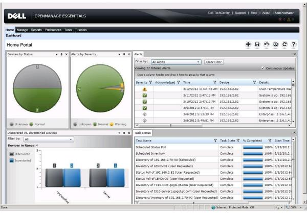
Figure 8. Dell OpenManage Essentials dashboard view showing temperature alert on the TS430.
