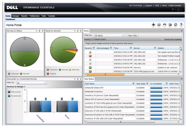
Figure 5. Dell OpenManage Essentials dashboard view of fan alerts on the TS430.
