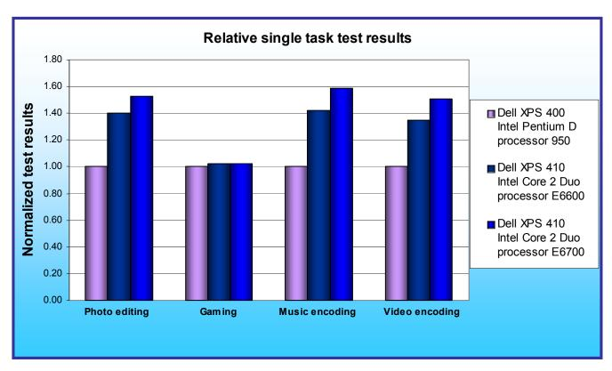
Figure 1: Relative single-task results for Dell XPS 400-series systems with various Intel processors on the customized tests.
