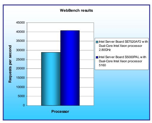
Figure 1: Peak (dual processor) performance of the test servers running WebBench 5.0. Higher numbers of requests per second are better.
