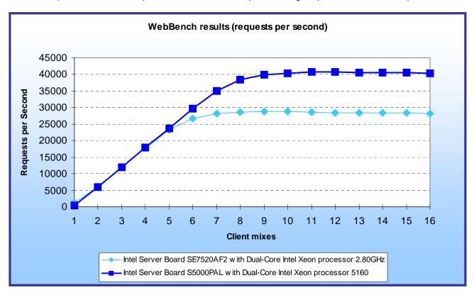
Figure 3: Line graph of the WebBench requests per second results for the two test servers. A higher peak indicates better performance.
