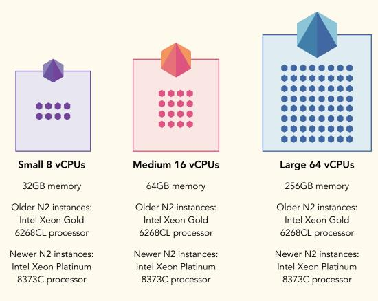
Figure 1: Key specifications of the Google Cloud N2 instances we tested. Source: Principled Technologies.
