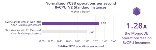
Figure 2: Comparison of the rate at which each of the small N2 instances featuring 3<sup>rd</sup> Gen Intel Xeon Scalable processors completed the MongoDB workload, relative to the rate of the N2 instances with older processors. Higher is better. Source: Principled Technologies.
