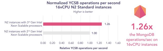
Figure 3: Comparison of the rate at which each of the medium N2 instances featuring 3<sup>rd</sup> Gen Intel Xeon Scalable processors completed the MongoDB workload, relative to the rate of the N2 instances with older processors. Higher is better. Source: Principled Technologies.
