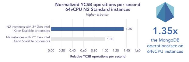
Figure 4: Comparison of the rate at which each of the large N2 instances featuring 3<sup>rd</sup> Gen Intel Xeon Scalable processors completed the MongoDB workload, relative to the rate of the N2 instances with older processors. Higher is better. Source: Principled Technologies.
