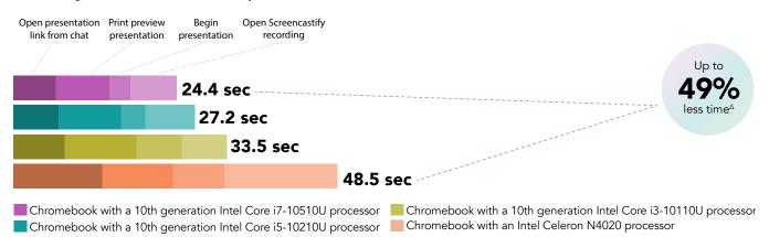
Figure 3: Time (in seconds) to complete a series of tasks while also engaging in a five-way video chat session in Google Meet. Less time is better. Source: Principled Technologies.
