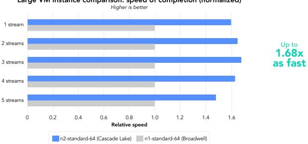
Large VM instance comparison: speed of completion (normalized)
