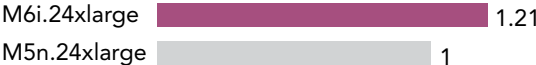
Figure 3: Relative number of frames per second that the large M6i and M5n instances (96 vCPUs) handled using the ResNet50 benchmark. Higher numbers are better. Source: Principled Technologies.
