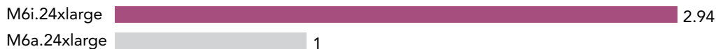
Figure 5: Relative number of frames per second that the large M6i and M6a instances (96 vCPUs) handled using the ResNet50 benchmark. Higher numbers are better. Source: Principled Technologies.
