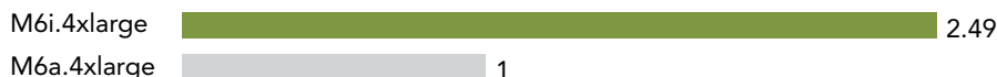
Figure 4: Relative number of frames per second that small M6i and M6a instances (16 vCPUs) handled using the ResNet50 benchmark. Higher numbers are better. Source: Principled Technologies.
