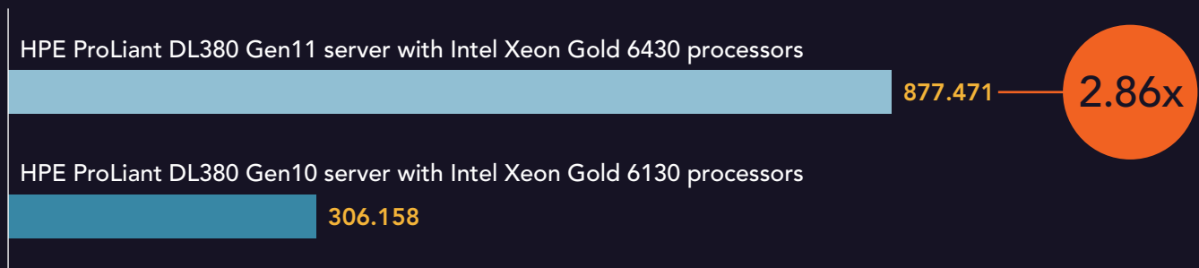
Figure 1: The number of images per second each server processed on the ResNet-50 v1.5 model with FP32 precision. Higher is better. Source: Principled Technologies.
