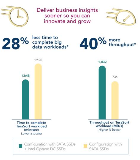
\*according to tests we conducted on the TeraSort benchmark, using a Hadoop cluster with HPE ProLiant DL380 Gen10 servers and Intel Optane DC SSDs, compared to the same server clusters using only SATA SSDs
