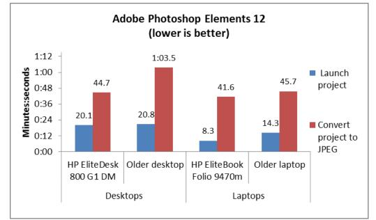
Figure 2: Time the four test systems needed to launch an Adobe Photoshop Elements 12 project and convert it to JPEG. Lower times are better.
