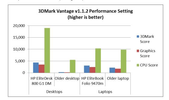
Figure 4: 3DMark Vantage v1.1.2 Performance Setting scores the four test systems achieved. Higher scores are better.
