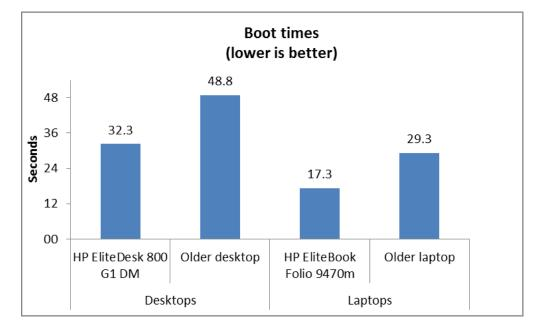
Figure 1: Time the four test systems needed to boot. Lower times are better.
