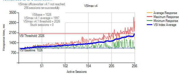
Figure 8: The legacy Cisco server using a traditional SAN with four B200 M2 blades ran 256 sessions and did not reach VSImax; Adding additional sessions caused the server to reach VSImax due to CPU saturation and unacceptable end-user response times.
