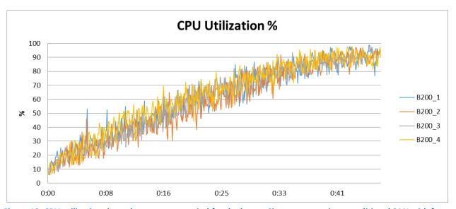
Figure 12: CPU utilization throughout our test period for the legacy Cisco servers using a traditional SAN with four B200 M2 blades with 256 VDI users.
