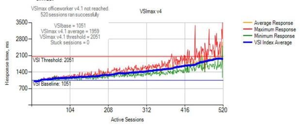
Figure 7: The Dell PowerEdge FX2 using VMware Virtual SAN with four FC430 sleds ran 520 sessions while maintaining acceptable end user response times. Adding additional sessions caused the server to reach VSImax due to CPU saturation.
