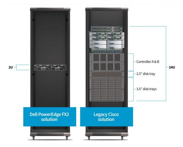
Figure 2: The space requirements of the Dell PowerEdge FX2 solution vs. the legacy Cisco solution.
