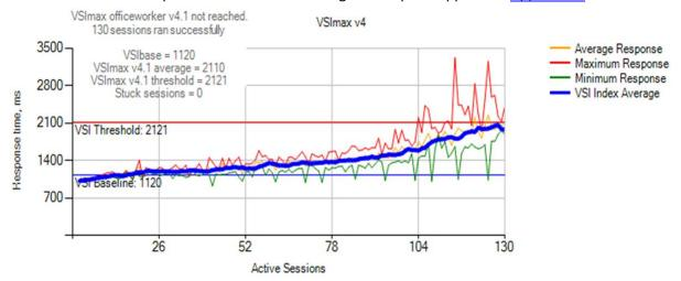
Figure 5: The Dell PowerEdge FX2 using VMware Virtual SAN with a single FC430 sled ran 130 sessions while maintaining acceptable end user response times. Adding additional sessions caused the server to reach VSImax due to CPU saturation.
