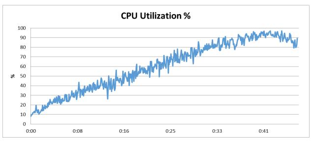
Figure 9: CPU utilization throughout our test period for the Dell PowerEdge FX2 using VMware Virtual SAN with one FC430 sled with 130 VDI users.
