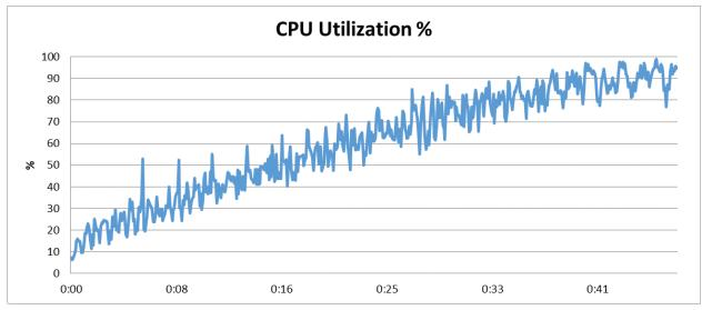
Figure 10: CPU utilization throughout our test period for the legacy Cisco server using a traditional SAN with one B200 M2 blade with 64 VDI users.
