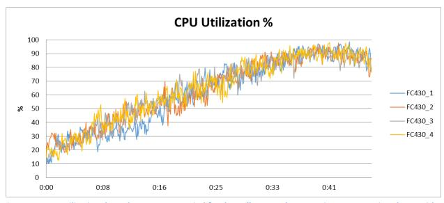
Figure 11: CPU utilization throughout our test period for the Dell PowerEdge FX2 using VMware Virtual SAN with four FC430 sleds with 520 VDI users.
