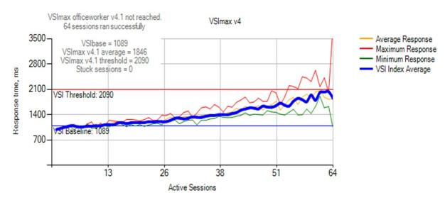
Figure 6: The legacy Cisco server using a traditional SAN with a single B200 M2 blade ran 64 sessions and did not reach VSImax. Adding additional sessions caused the server to reach VSImax due to CPU saturation.
