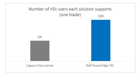
We then increased the number of FC430 server sleds running the VDI workload in the Dell PowerEdge FX2 and the number of blades on the legacy Cisco solution running the same workload to four, and found that performance scaled evenly, supporting 520 and 256 sessions respectively (see Figure 4).
