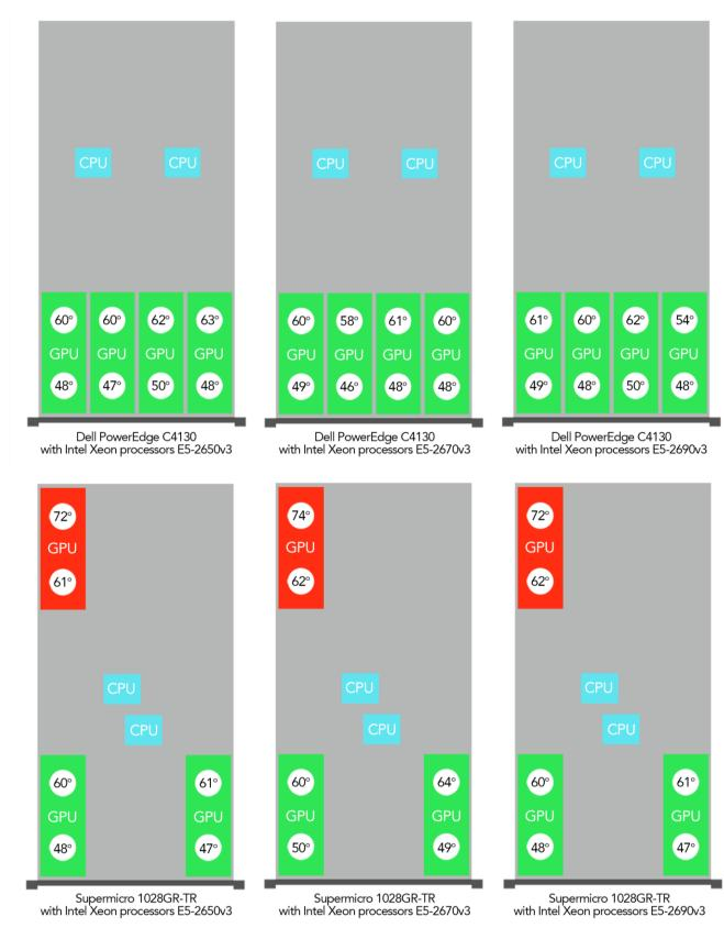
Figure 4: GPU and CPU placement in the two servers we tested showing sensor temperatures with multiple Intel Xeon processor configurations.
