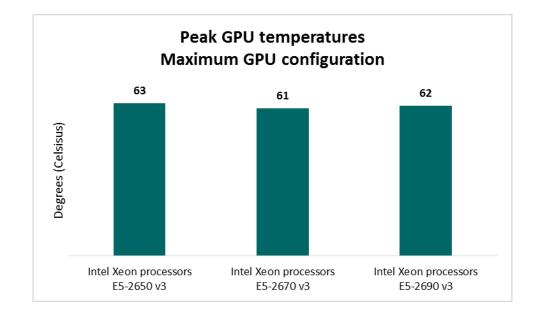
Figure 3: Peak GPU temperature for the maximum configurations of the Dell PowerEdge C4130 with each of the three Intel Xeon processors.
