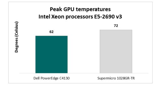
Figure 10: Peak GPU temperature for the maximum configuration of both systems. Lower numbers are better.
