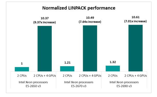
Figure 2: Normalized LINPACK floating-point performance for the baseline and maximum configuration of the PowerEdge C4130 using multiple Intel Xeon processor configurations. Higher numbers are better.
