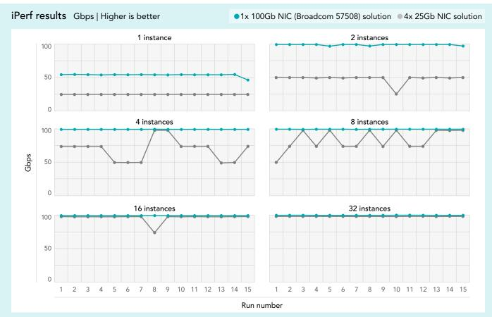
Figure 1: iPerf results, in Gbps, for the two NIC solutions. Higher numbers are better. Source: Principled Technologies.
