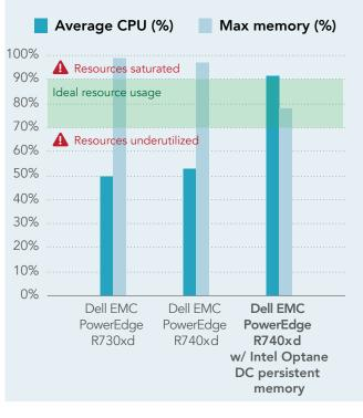
memory saturation would cause VDI user sessions to slow, freeze, and ultimately cease functioning. Intel Optane DC persistent memory enabled the PowerEdge R740xd to use just under 80 percent of its memory and around 90 percent of its CPU—a much better balance that enabled the server to take full advantage of its resources. The result in our tests was an increase of up to 3.75 times the number of VDI users, a figure that could help you get more from your data center investment.
