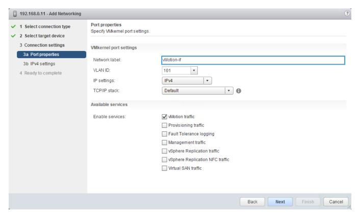
Figure 19: Enabling vMotion traffic and setting the appropriate VLAN ID on a new VMkernel port.
