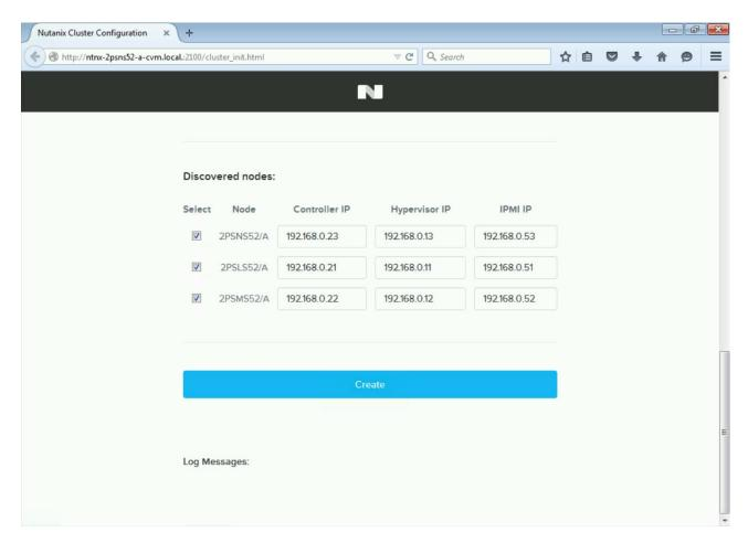
Figure 8: Provide IP addresses for the Controller, Hypervisor, and IPMI for each discovered node.
