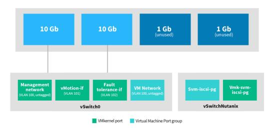
Figure 4: The structure of each XC630 host's NIC team, formed from the two 10 Gbps ports, and their virtual switches and VMkernel ports and port groups. Note that the 1 Gbps ports are unused.
