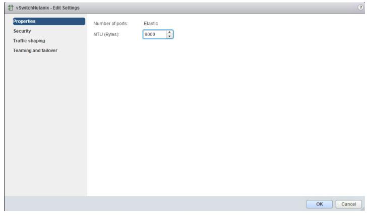
Figure 20: Enabling jumbo frames (MTU 9000) on the Nutanix vSwitch.
