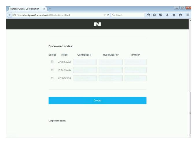
Figure 7: If IPv6 link-local connectivity is working properly, your nodes should appear in the list of Discovered nodes.
