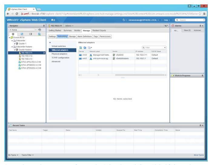
Figure 18: The network management page for an XC30 host in the vSphere Web Client, with the default network configuration.
