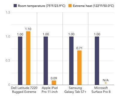
Figure 1: Geekbench 5 CPU performance scores in high heat normalized to scores at room temperature. Higher is better. Source: Principled Technologies.
