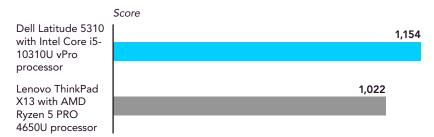
Figure 4: SYSmark 2018 overall performance rating while running on battery. Higher is better. Source: Principled Technologies.
