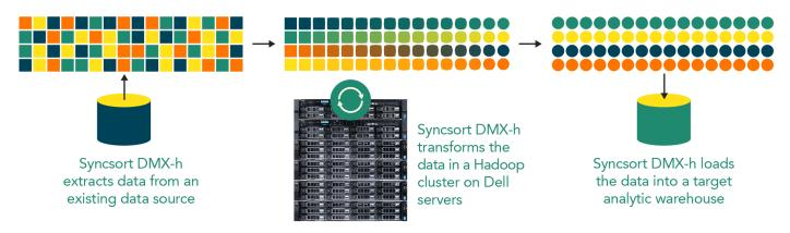
Figure 2: How the Dell | Cloudera | Syncsort solution for Hadoop works.
