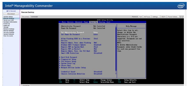
Figure 3: Editing BIOS settings via Intel AMT
