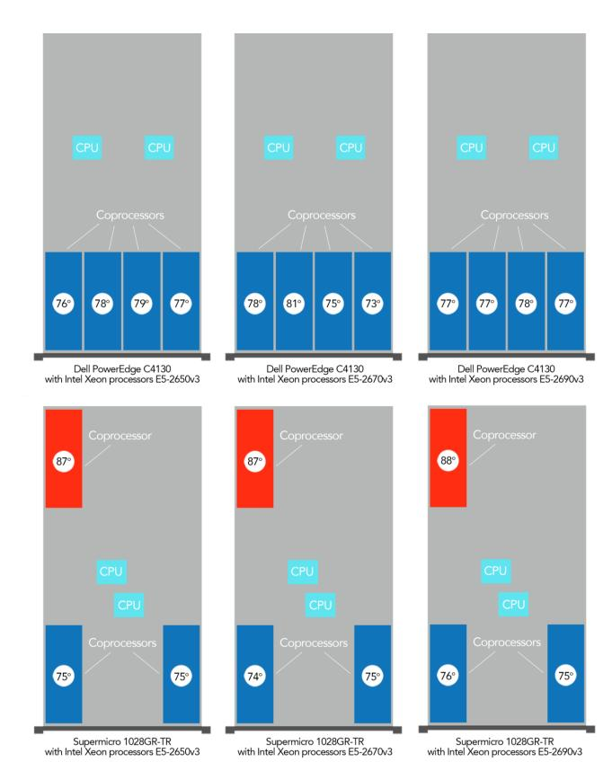
Figure 4: Coprocessor and CPU placement in the two servers we tested showing sensor temperatures with multiple Intel Xeon processor configurations. Lower temperatures are better.
