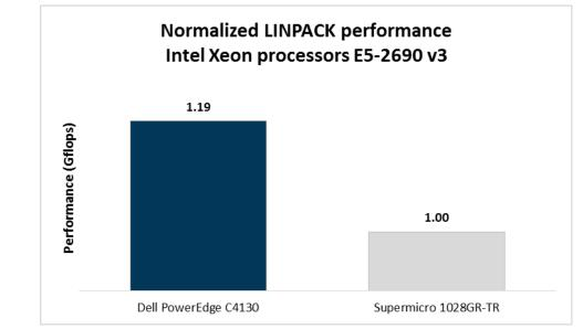
Figure 9: Normalized LINPACK floating-point performance for each system. Higher numbers are better.
