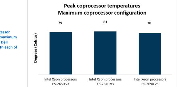
Figure 3: Peak coprocessor temperature for the maximum configurations of the Dell PowerEdge C4130 with each of the three Intel Xeon processors.
