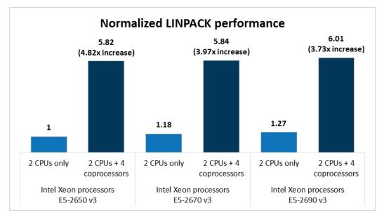
Figure 2: Normalized LINPACK floating-point performance for the baseline and maximum configuration of the PowerEdge C4130 using multiple Intel Xeon processor configurations. Higher numbers are better.
