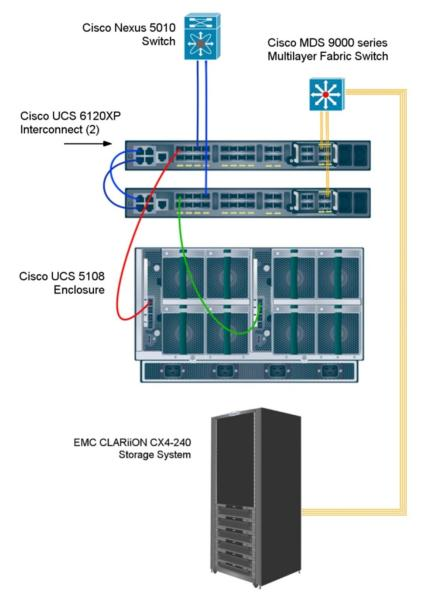
Figure 6: Our test bed configuration for the Cisco UCS B250 M1 Extended Memory Blade Server.
