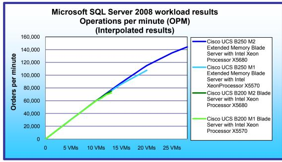
Figure 2: Blade server comparison results in operations per minute. Higher numbers are better.
